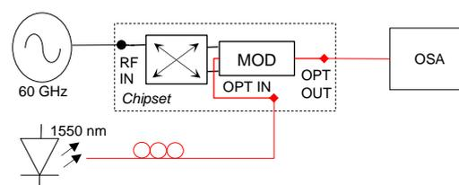
Fig. 3: Experimental setup for single-tone modulation characterization.
