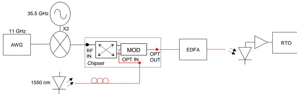
Fig. 5: Experimental setup for link experiments.
