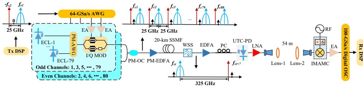
Fig. 1: Principle and experimental setup of THz-wave signal wireless transmission in an 80-channel WDM system.
