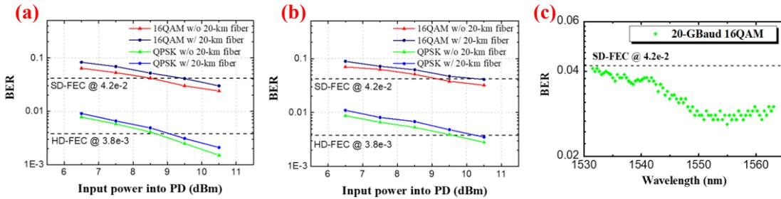
**Fig. 4:** BER versus input power into PD for 20-Gbaud 16QAM and QPSK signals (a) @ 1563.05 nm and (b) @ 1531.51 nm w/o and w/ 20-km fiber transmission before 54-m wireless transmission. (c) BER of all 80 channels 20-Gbaud 16QAM THz-wave signals after 20-km fiber transmission and 54-m wireless transmission.
