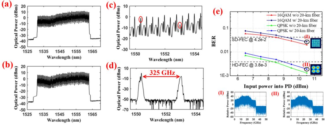
**Fig. 3:** Optical spectra of 80-channel 20-Gbaud 16QAM signals (a) w/o and (b) w/ 20-km fiber transmission. Optical spectra of 20-Gbaud 16QAM signal with 325GHz space (c) before and (d) after WSS. (e) BER versus input power into PD for 20-Gbaud 16QAM and QPSK signals @ 1553.33 nm w/o and w/ 20-km fiber transmission before 54-m wireless transmission. Insets (I) and (II) are electrical spectra of the received 20-Gbaud 16QAM and QPSK IF signals, respectively.
