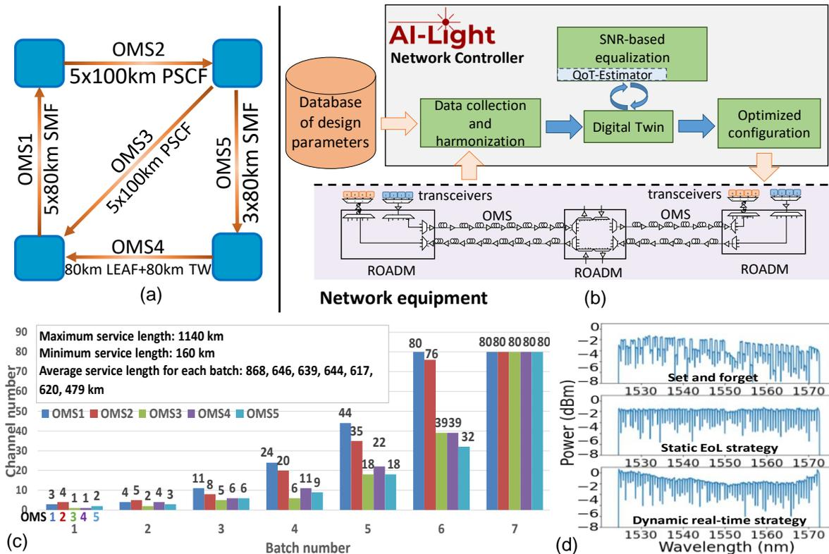
**Fig. 1:** (a) Topology of the experimental mesh network; (b) AI-Light SDN framework; (c) Number of services transported by each OMS after loading each batch; (d) Full-load normalized power spectrum for each power re-optimization strategy.
