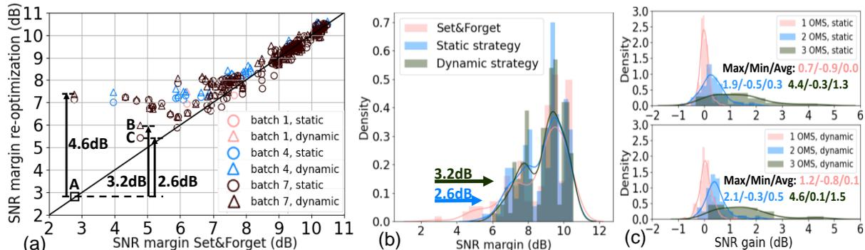
**Fig. 3:** (a) SNR of services with power re-optimization strategies vs. “set and forget”; (b) PDF of SNR margins; (c) PDF of SNR gain per length (1, 2, 3 OMS) and per power re-optimization strategy.
