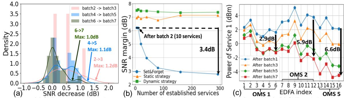
**Fig. 2:** (a) SNR decrease of existing services (batch  $N$ ) due to loading new services (batch  $N+1$ ); (b) SNR variation of Service 1 with different number of established services; (c) Power of Service 1 after each traversed EDFA.
