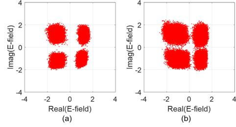
**Fig. 7:** Measured QPSK constellations at (a) 40 GBaud and (b) 50 GBaud, both with FFE applied to the IQ-MZI. The measured voltage swings are 60 mVpp and 80 mVpp for 40 GBaud and 50 GBaud, respectively.
