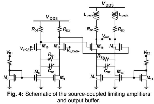
**Fig. 4:** Schematic of the source-coupled limiting amplifiers and output buffer.
