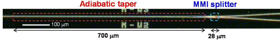
Fig. 4: Microscopic image of the fabricated PSR on InP.
