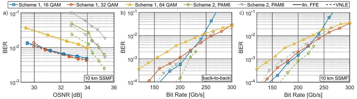
**Fig. 3:** Experimental results. a) shows the BER as a function of the OSNR for a bit rate of 224/225 Gb/s and 10 km transmission in C-band. b) and c) show the comparison of both schemes for rates between 120 Gb/s and 300 Gb/s for back-to-back and 10 km SSMF transmission. The solid curves were obtained based on linear FFE and the dashed curves on VNLE.
