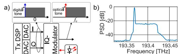
**Fig. 1:** a) transmitter configuration for SSB signal generation using a virtual carrier and b) exemplary optical spectrum of a resulting signal.
