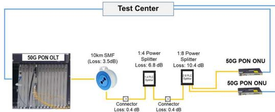
Figure 7: Carrier lab trial test configuration
