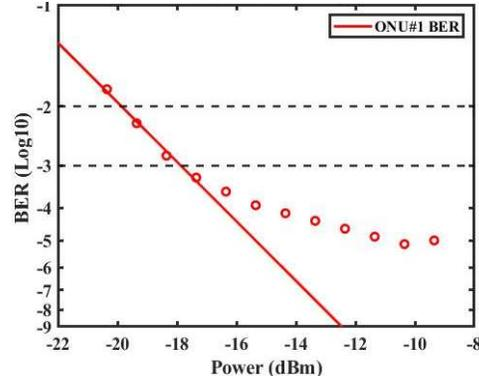
Fig. 5 BER vs received power at the ONU.
