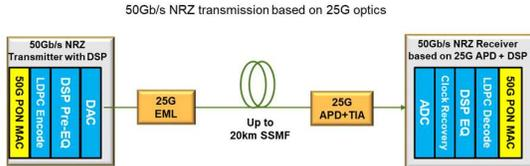
Figure 2: 50Gbps NRZ transmission based on 25G-class optics for 50G-PON downstream
