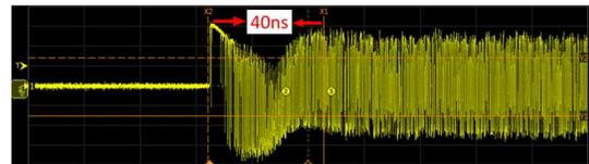
Fig. 6: 25Gbps Burst-mode upstream signal reception
