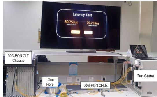
Figure 8: Latency measurement in carrier lab trial
