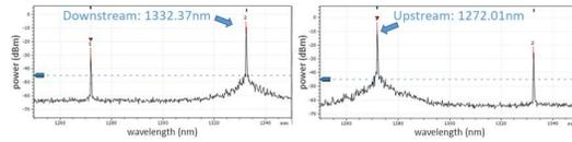
Fig. 4 Optical spectra for (a) DS signal and (b) US signal.
