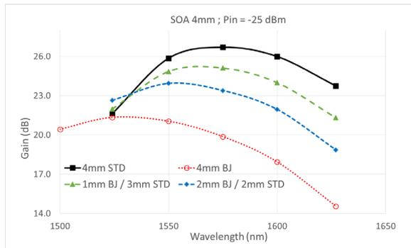
**Fig. 4:** Measured gain of 4 mm long SOA, made with 0, 1, 2 or 4 mm of BJ material.
