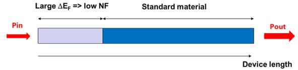
Fig. 3: Top-view of proposed low NF SOA design
