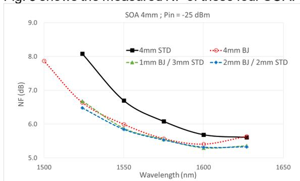
**Fig. 5:** Measured NF of 4 mm long SOA, made with 0, 1, 2 or 4 mm of BJ material, and the rest with standard material.
