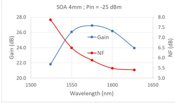
Fig. 1: Measured gain and NF of a 4 mm long SOA
