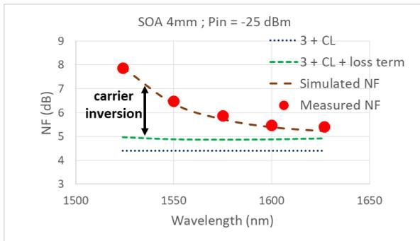
Fig. 2: Calculated and measured NF of a 4 mm long SOA
