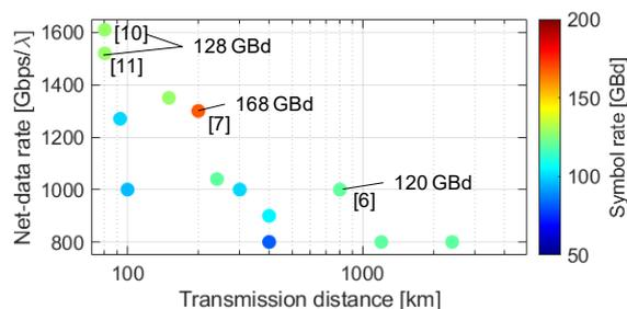
Fig. 1: Net-data rate per wavelength as a function of transmission distance
