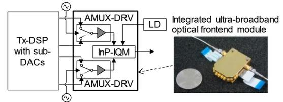
**Fig. 4:** High speed optical transmitter based on integrated ultra-broadband optical frontend module
