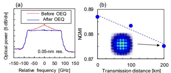
**Fig. 5:** Experimental results of 1.3-Tbps PCS-64QAM: (a) optical spectra before/after OEQ and (b) NGMI versus transmission distance (NGMI limit: 0.857)
