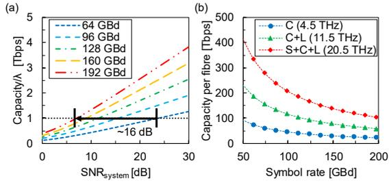
**Fig. 2:** Achievable capacity: (a) capacity per wavelength versus SNR in each symbol rate and (b) capacity per fibre versus symbol rate in 1-Tbps/λ WDM system.
