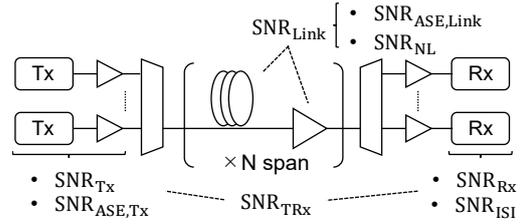
**Fig. 3:** System model of optical transmission.
