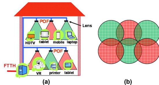
**Fig. 1:** An in-home network employing luminaire-free LiFi transmission systems using POF and lens (a) and footprint of the luminaires showing partly overlapped areas (b).
