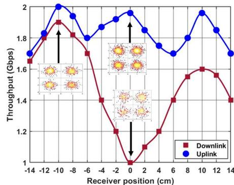
Fig. 4: Link performance of the VLC transmission with WDM over-POF for downlink and uplink applying DMT modulation.
