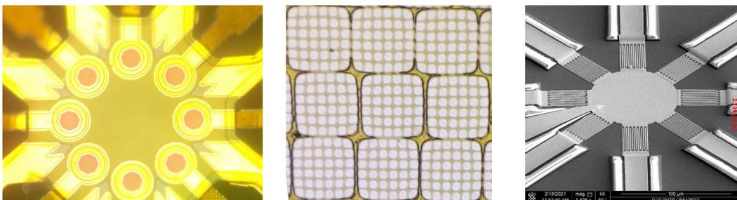
**Fig. 1:** Components for the link. Left: 8 element emitter array. Center: imaging fiber consisting of 9 elements of 6x6 with 10 $\mu$ m cores – note each lane is carried by a few adjacent cores. Right: 8 element lateral p-i-n detector array
