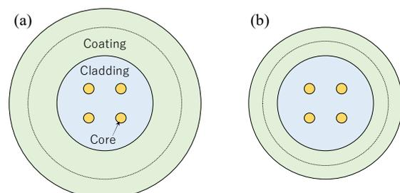
**Fig. 1:** Schematics of cross-section of prepared 4CFs (a) 250-4CF and (b) 200-4CF.
