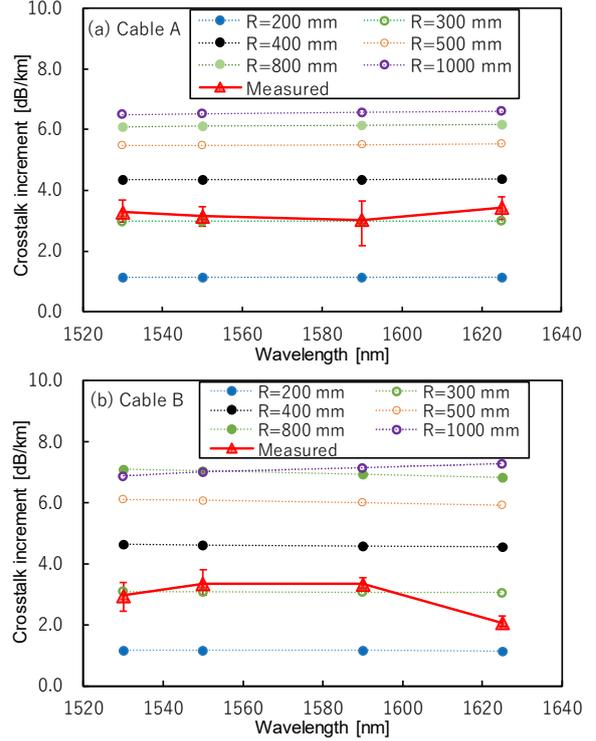
**Fig. 6:** Crosstalk increment after cabling as compared to before cabling for (a) Cable A (200-4CFs) and (b) Cable B (250-4CFs). Fibre spool radius of 4CFs before cabling was 155 mm.
