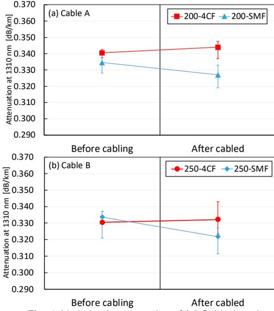
**Fig. 4:** Variation in attenuation of (a) Cable A and (b) Cable B at 1310 nm.
