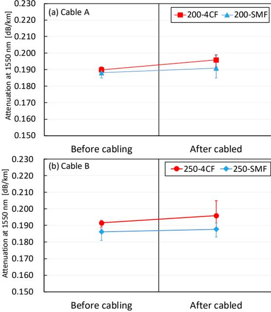
**Fig. 5:** Variation in attenuation of (a) Cable A and (b) Cable B at 1550 nm.
