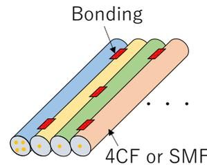
**Fig. 2:** Schematic diagram of the fabricated intermittently bonded optical fibre ribbon.
