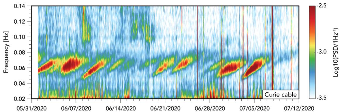
**Fig. 1:** Spectrogram of the SOP modulation recorded over the Curie cable in June-July 2020. Energy dispersion around 60mHz is clearly visible and can be associated with primary microseism caused by ocean swells.
