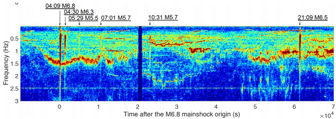
**Fig. 1:** SOP signals of the 01 September 2020 M6.8 submarine earthquake offshore Chile. Five of the largest aftershocks (between M6.5 and M5.5) can be clearly identified as vertical wavepackets in the spectrogram
