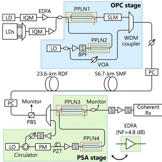
**Fig. 1:** Experimental setup. LD: laser diode, IQM: I/Q modulator, VOA: variable optical attenuator, PC: polarisation controller, PBS: polarisation beam splitter, PZT: piezoelectric transducer-based fibre stretcher, BPF: band-pass filter, LO: local oscillator, PM: phase modulator.
