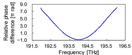
**Fig. 3:** Calculated relative phase difference from locking frequency due to residual CD.
