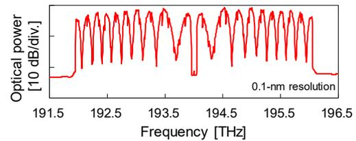
**Fig. 2:** Spectrum of WDM signal after phase-sensitive amplification without CD pre-compensation.
