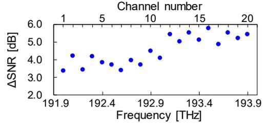
Fig. 6:  $\Delta$ SNR characteristic indicates SNR improvement amount by PSA in each channel.
