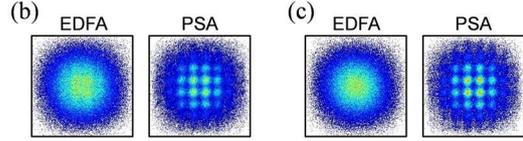
Fig. 5: Received signal characteristics. (a) NGMIs of 20-ch. 96-Gbaud SP-PS-64QAM signals. Constellation diagrams of (b) ch.1 and (c) ch.20.
