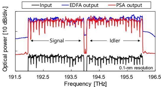
Fig. 4: WDM spectra after pre-amplifying by PSA or EDFA.
