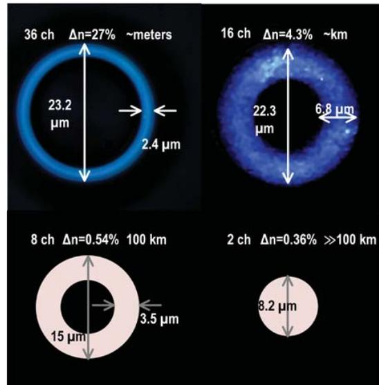
Fig. 1: Enhanced scanning electron microscope photos of upper left: air core RCF<sup>[10]</sup>, upper right: thick core RCF with high contrast<sup>[12]</sup>; and cartoons of fibers in lower left: thick core RCF with low contrast<sup>[8]</sup>, lower right: typical SMF with low contrast
