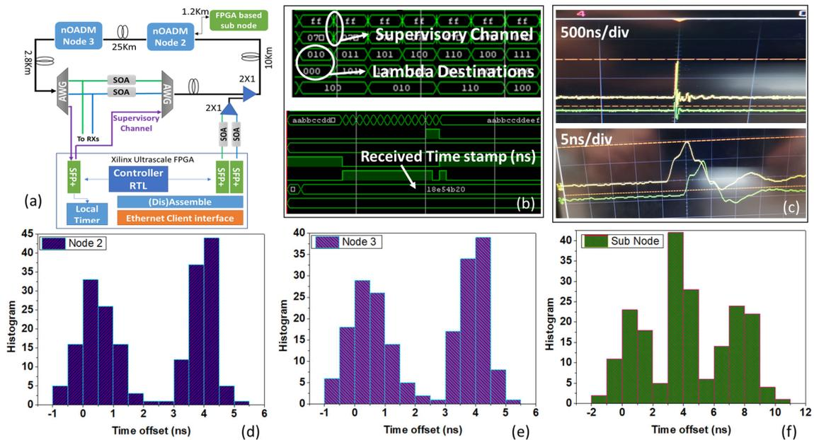
**Fig. 2:** (a) Experiment setup; (b) FPGA trace of the supervisory channel and received time stamp of master node; (c) gap between two PPS signal of master node and node 2; (d) Histogram of the time offset between master node and node 2; (e) Histogram of the time offset between master node and node 3; (f) Histogram of the time offset between master node and sub node.
