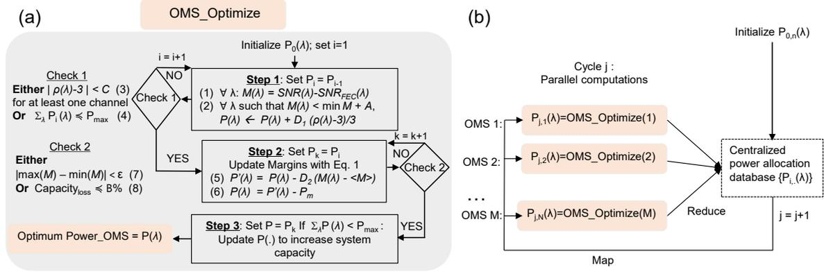
Fig. 1: (a) Single OMS power optimization algorithm "OMS\_Optimize"; (b) Network-wide power equalization algorithm.
