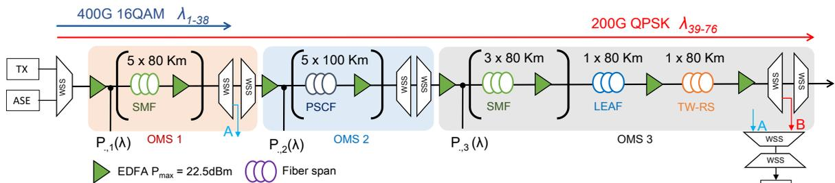
Fig. 2: Experimental Setup: 3 OMS, 76 channels.
