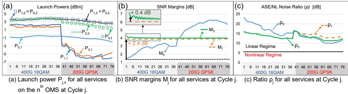
**Fig. 3:** Simulations: equalization of a 3-OMS network.
