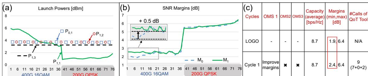
**Fig. 4:** Experiment: (a) launch powers  $P_{j,n}$  for all services on  $n^{\text{th}}$  OMS at Cycle  $j$ ; Margins  $M_j$  at Cycle  $j$ ; (c) Cycles.
