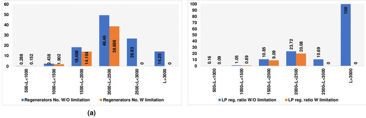
**Fig. 3:** The (a) regenerators quantity, and (b) LP regenerator assignment ratio, for a range of different route lengths within the USNET topology.
