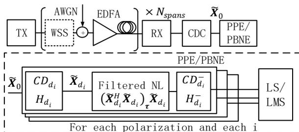
**Fig.1:** Block diagram of VNLE-based PPE/PBNE.
