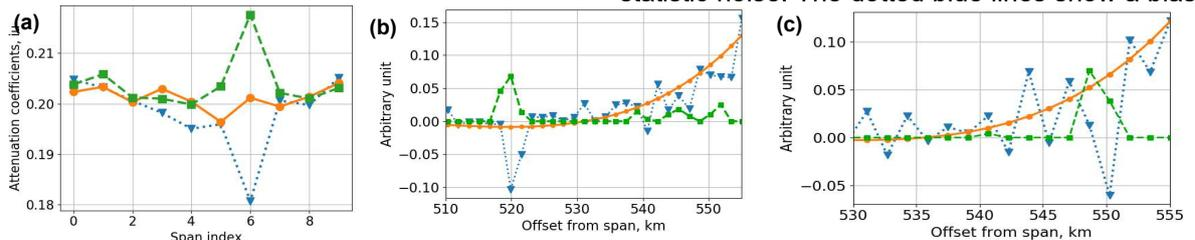
**Fig.3:** (a) Attenuation estimation for an abnormal attenuation added to 6th span fiber. For solid orange, dotted blue and dashed green curve, set attenuation are 0.2, 0.18 and 0.22 dB/km, respectively. (b, c) Abnormal loss estimation for 1 dB loss at 520 km (b) and 550 km (c) point. Dotted blue, solid orange and dashed green curves present  $\Delta$ ,  $\zeta_{est}$  and bias corrected estimation, respectively.
