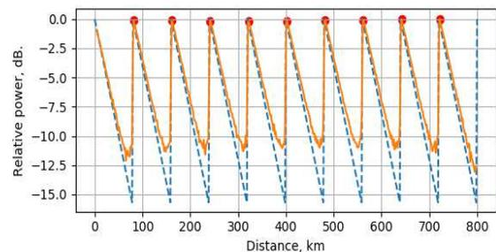
**Fig.2:** PP estimation. Solid line is the estimated PP and dashed line is the real transmitted PP.
