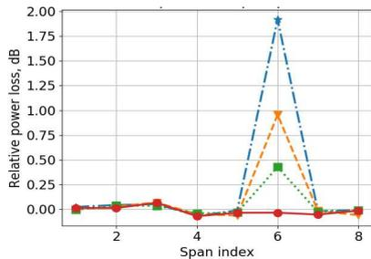
**Fig.4** Power loss in EDFA at the end of 6th span. Set gain loss for solid red, dotted green, dashed orange and dashed-dotted blue line are estimation from the simulation with 0.0, 0.5, 1.0, 2.0 dB loss, respectively.
