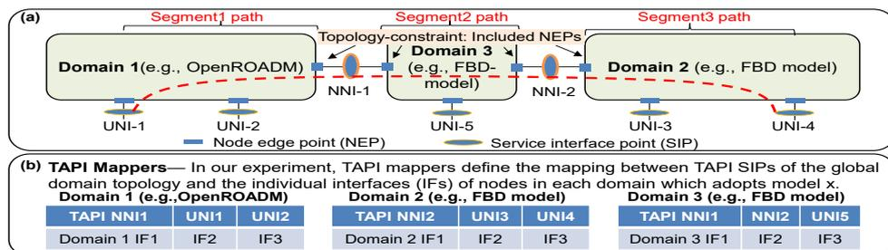
Fig. 3: TAPI topology/mappers in integration/control of heterogenous optical networks spanning from Telecom to DC. (a) TAPI topology of heterogenous domain with different device/network models, (b) TAPI mappers of individual networks
