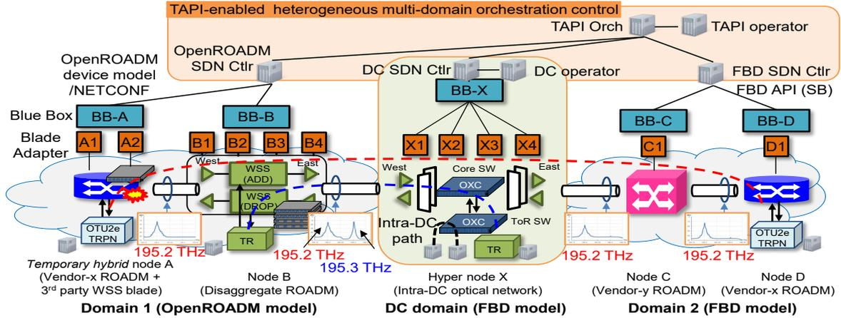
**Fig. 4:** Experiment of integration/control of heterogeneous Telecom and DC optical networks aided by TAPI and FBD
