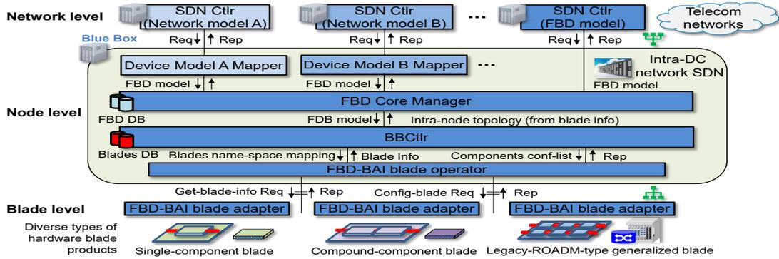
Fig. 2: Unified FBD-based nodal structure in Telecom and DC optical networks
