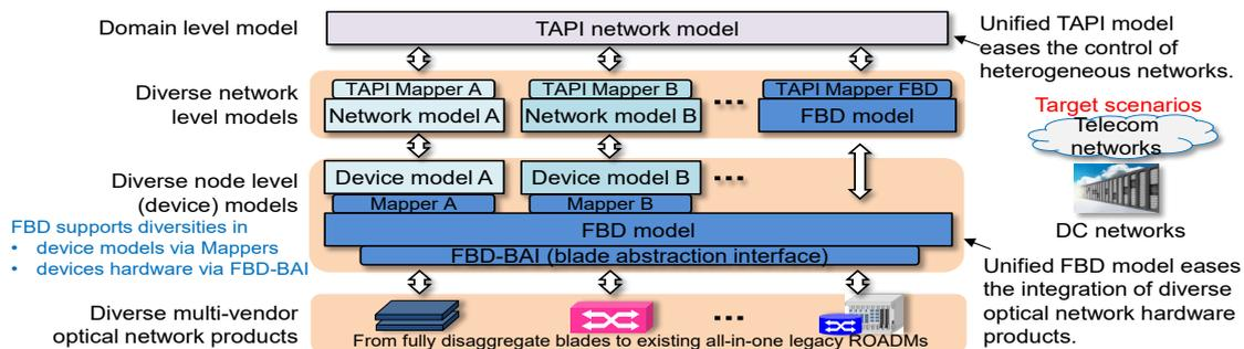
Fig. 1: Reference model for integration/control of heterogeneous Telecom/DC optical networks aided by FBD-BAI & TAPI
