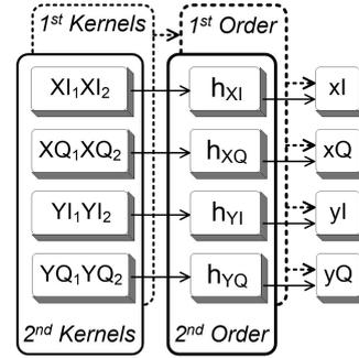
**Fig. 3:** Principle of VNLE scheme.
