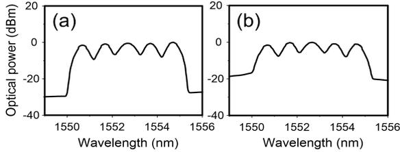
**Fig. 2:** The optical spectra of 5-channel WDM PS-16QAM signals (a) before and (b) after 6,400-km transmission.
