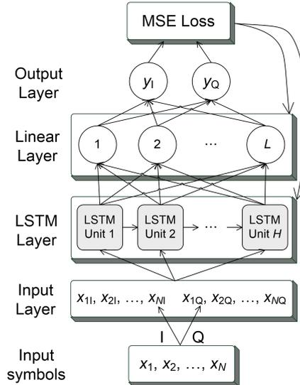
**Fig. 4:** Structure of modified LSTM-NLE.
