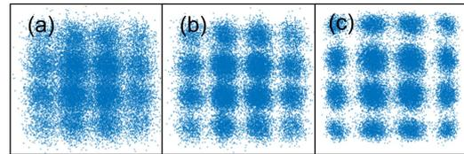
Fig. 7: Constellations (a) before NLE, (b) after VNLE and (c) after LSTM-VNLE.
