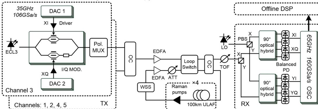
Fig. 1: Experimental setup of 5-channel WDM transmission based on 106-Gbaud PM PS-16QAM.
