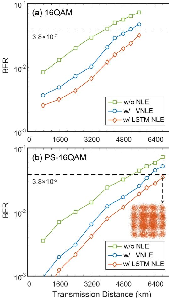
Fig. 6: BER versus ULAH transmission distance.
