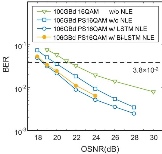
Fig. 5: BER versus OSNR under BtB condition.
