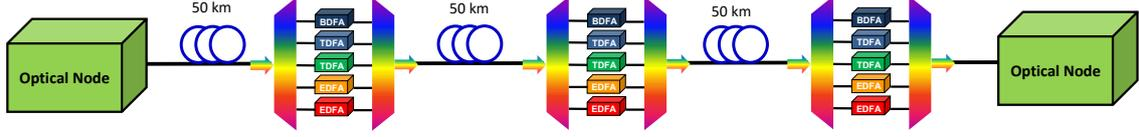
Fig. 1: The transmission link used to interconnect two consecutive nodes
