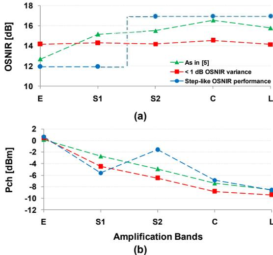
Fig. 2: OSNIR for different amplification bands using three different power allocation schemes
