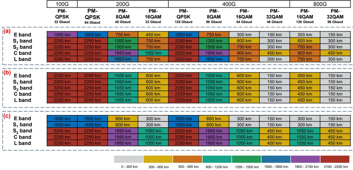
Fig. 3: Attainable reach for three optimization methods to: (a) balanced OSNIR between different bands, (b) flat OSNIR between all bands, (c) flat OSNIR within two zones.
