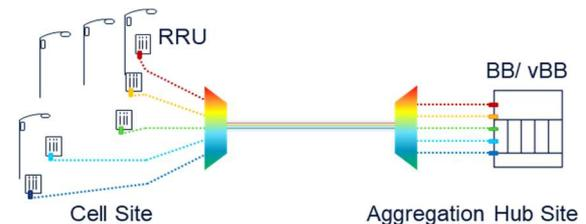
Fig. 1: Passive-passive Optical WDM Fronthaul network
