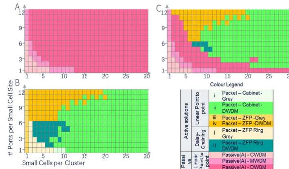
**Fig. 6:** Lowest TCO Heat map for (A) Passive-only, (B) Active-only, (C) Passive and Active architectures.
