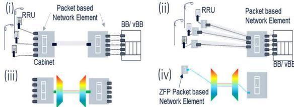
**Fig. 2:** Active-active Packetized Fronthaul network architectures
