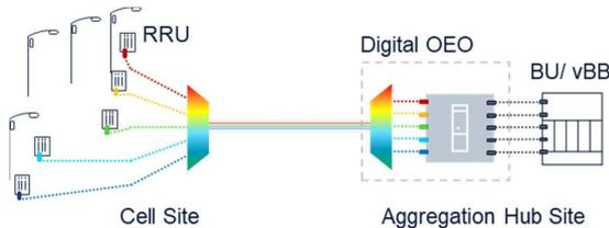
**Fig. 3:** Semi-active Optical WDM Fronthaul network
