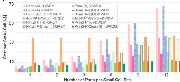
**Fig. 5:** Solution cost per cell site as a function of port count.
