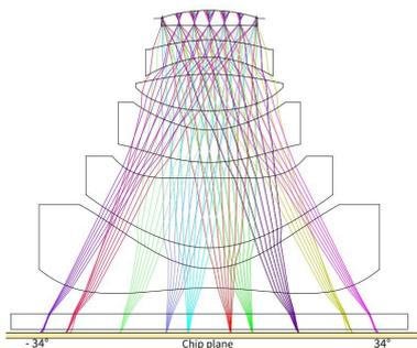
**Fig. 7:** Camera lens system for the chip.
