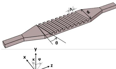
**Fig. 1:** Schematic of tilted grating coupler.  $\theta$  is the tilted angle of the grating teeth and  $\Lambda$  is the period.  $\kappa$  zenith direction of radiation and  $\phi$  azimuth direction of radiation
