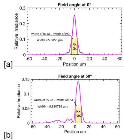
**Fig. 9:** a)FWHM of PSF at 0 degrees. b) FWHM of PSF at 50 degrees.
