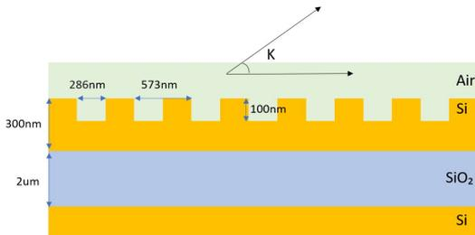
**Fig. 3:** Illustration of the slanted GC waveguide structure.
