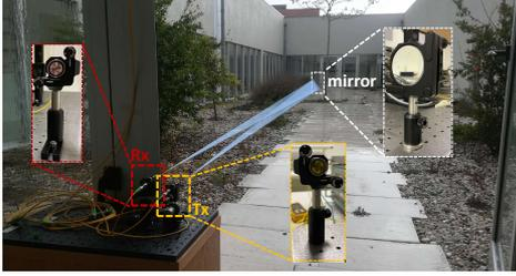
**Fig. 3:** Outdoor FSO link for 400G+ transmission enabled by adaptive modulation.
