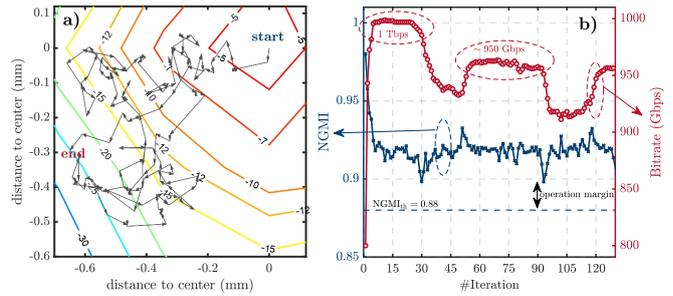
**Fig. 7:** Experimental demonstration of Terabit-capable FSO transmission for intra-DC transmission. a) emulated impact of pointing errors; b) adapted bit-rate and NGMI over time.
