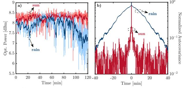
**Fig. 4:** Impact of atmospheric turbulence and weather phenomena on FSO power budget. a) received optical power over time with sun and rain conditions; b) normalized autocovariance unveiling the presence of time correlation.
