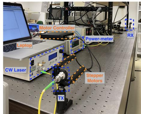
Fig. 1: Experimental setup with automatic beam alignment apparatus.
