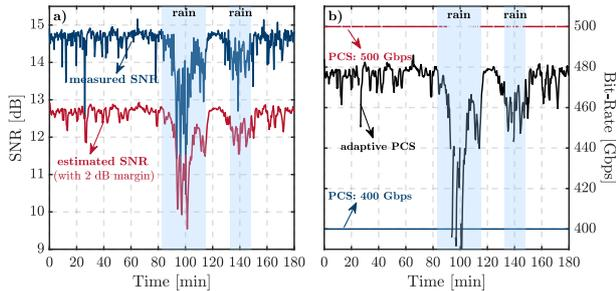
**Fig. 6:** Experimental demonstration of outdoor 400G+ FSO transmission with adaptive PCS modulation. a) measured and estimated SNR over time; b) bit-rate over time with fixed and adaptive PCS solutions.
