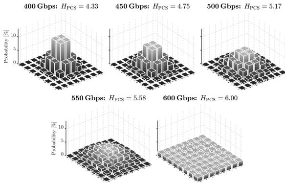
**Fig. 5:** PCS-64QAM configurations to deliver net bit-rates in the range of 400–600 Gbps for a fixed symbol-rate of 60 Gbaud,  $R_{FEC} = 5/6$  and  $R_{pil} = 1$ .
