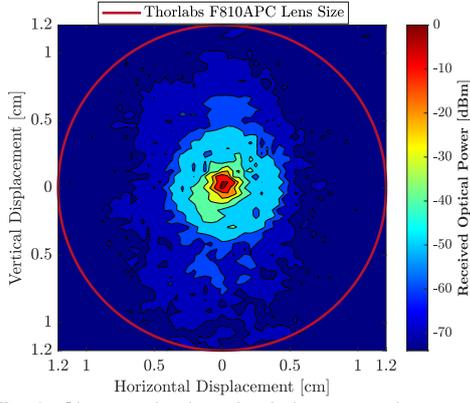
**Fig. 2:** Characterization of pointing error tolerance of Thorlabs F810APC fiber collimator.
