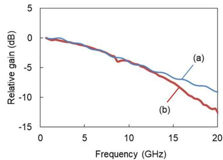
Fig. 5 Measurement results on (a) single PD and (b)  $8 \times 8$  PDA.
