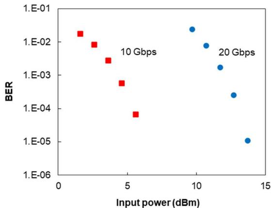
Fig. 7 BER measurement results with optical input power at (a) 10 Gbps (square), and (b) 20 Gbps (circle)
