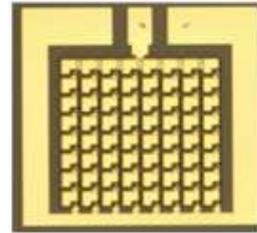
Fig. 4 Photograph of the fabricated  $8 \times 8$  PDA.
