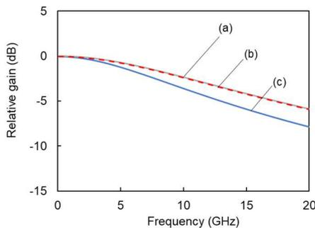
Fig. 3 Simulated frequency response: (a) single PD, (b)  $8 \times 8$  PDA, and (c)  $8 \times 8$  PDA with a shunt resistor.
