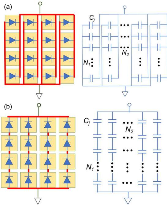
Fig. 2 (a) Model A using parallel connection and its equivalent circuit. (b) Model B using series connection.
