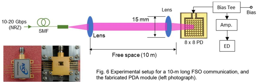
Fig. 6 Experimental setup for a 10-m long FSO communication, and the fabricated PDA module (left photograph).
