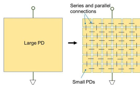
Fig. 1 Design concept of large high-speed PD.
