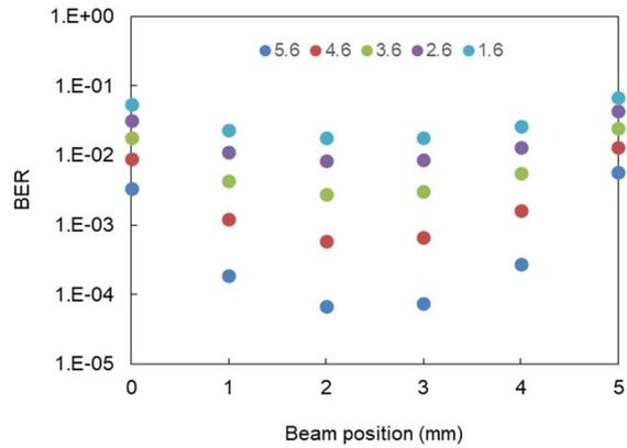
Fig. 8 BER at 10 Gbps when the beam position in 10-m free space is changed, with different input power levels (5.6/4.6/3.6/2.6/1.6 dBm)
