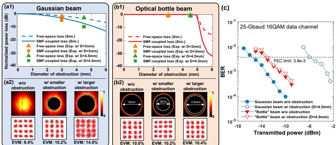
Fig. 3: Simulated and experimentally measure free-space and SMF-coupled power loss for the Gaussian (a1) and bottle beam (b1). Sim.: simulation; Exp.: experimental. Experimentally measured beam profiles and the EVM performance of the data signal w/ and w/o obstructions for the Gaussian (a2) and bottle beam (b2). (c) BER performance for the Gaussian and bottle beams w/o and w/ the larger obstruction under different transmission optical power.
