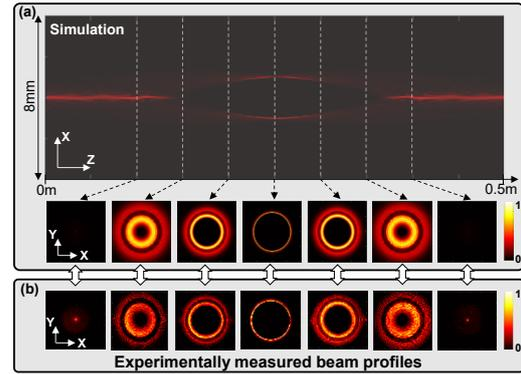
Fig. 2: (a) Simulated beam propagation and profiles of the bottle beam. (b) Experimentally measured beam intensity profiles of the generated bottle beam.
