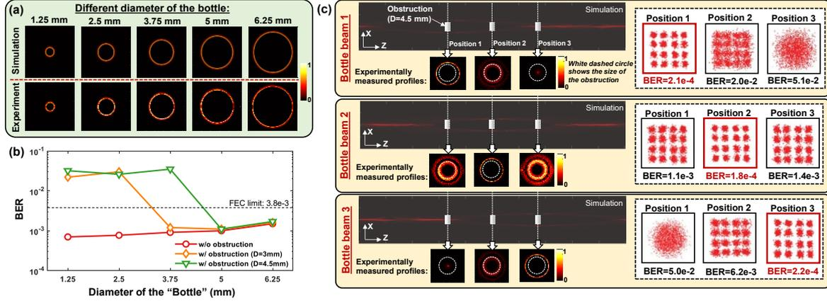
**Fig. 4:** (a) Simulated and experimentally measured profiles for bottle beams with different bottle sizes. (b) BER performance for bottle beams with different bottle sizes w/o and w/ obstructions. (c) Simulated beam propagation and experimentally measure profiles of bottle beams. Constellations and BER are measured w/ the obstruction located in different positions.
