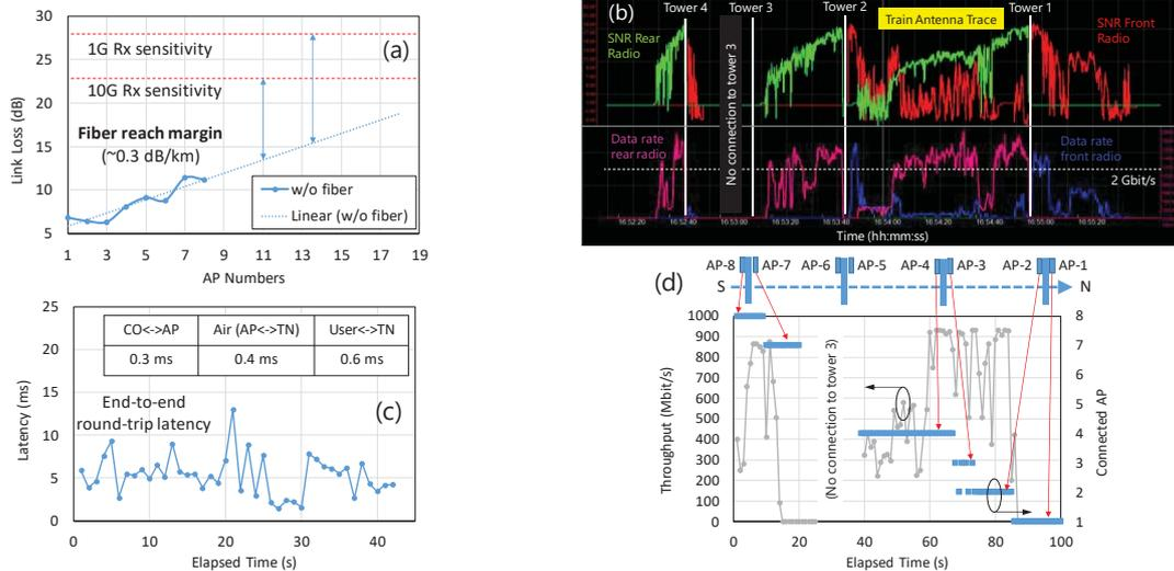
Fig. 3: (a) Link budget of passive add/drop WDM; (b) Mm-wave link telemetry; (c) End-to-end latency; (d) Handover analysis
