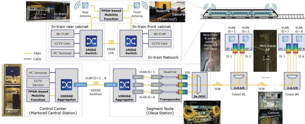
Fig. 2: Field trial setup composed of the control center, segment node, track-side network, and in-train network (inset photos)
