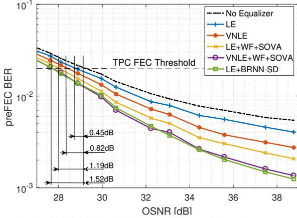
**Fig. 4:** 800G-96GBd-DP-32QAM optical BtB performance.
