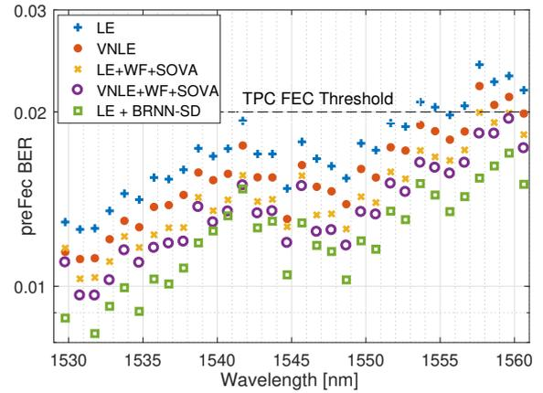
**Fig. 5:** 800G-96GBd-DP-32QAM Pre-FEC BER for the 32-channel DWDM system over a 600km G.654D fiber link.
