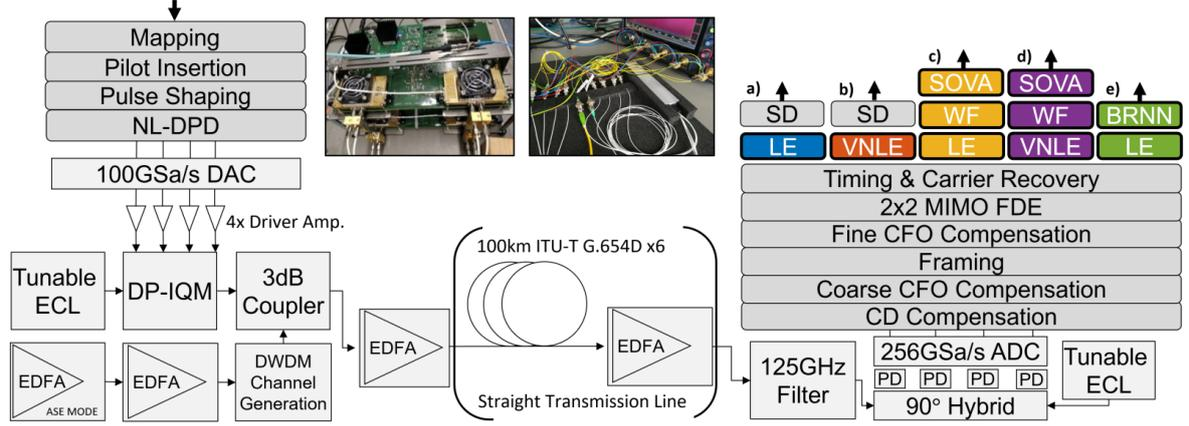
**Fig. 2:** Schematic of the DWDM experimental setup including the Tx and RX DSP architectures with a) Linear Equalizer (LE) & soft-demapper (SD) b) Volterra Equalizer (VNLE) & SD c) LE, whitening filter (WF) & accompanied by a soft-output Viterbi-algorithm (SOVA) d) VNLE, WF & SOVA and e) LE & BRNN soft-demapper.
