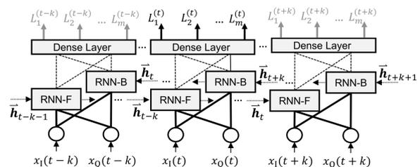
**Fig. 1:** BRNN Soft-Demapper: The final estimated soft information is provided by the centered dense output.
