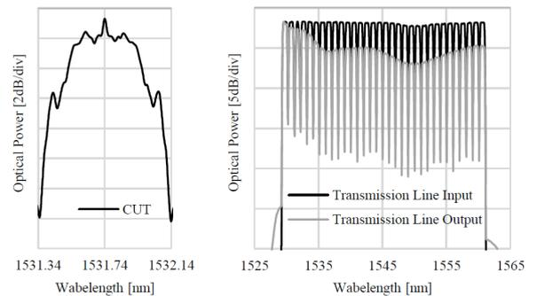
**Fig. 3:** DWDM experiment: spectrum of the 96GBd DP-32QAM CUT (left) and DWDM spectrum (right).
