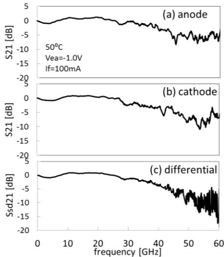
**Fig. 2:** Frequency response of (a) anode, (b) cathode, and (c) differential-drive conditions.
