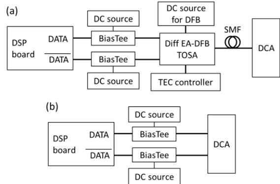
**Fig. 3:** Experimental setup for (a) DSP-direct differential drive of the fabricated differential EA-DFB TOSA and (b) measurement of intrinsic output from the DSP IC.
