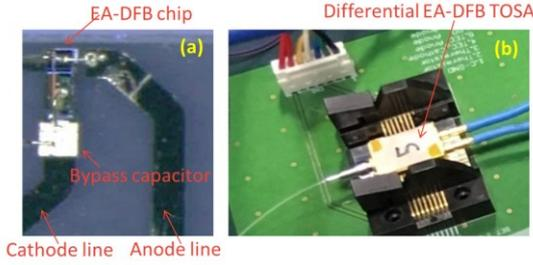
**Fig. 1:** Photograph of (a) EA-DFB on carrier developed for differential drive and (b) fabricated differential EA-DFB TOSA using the EA-DFB on carrier.
