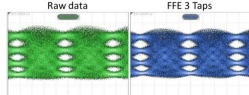
**Fig. 6:** Measured 53.125-Gbaud optical eye waveforms of raw data and with FFE of 3 taps with  $V_{ea}$  of -1.2 V and  $I_f$  of 100 mA at 50°C.
