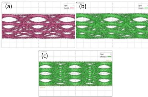
**Fig. 4:** 53.125-Gbaud electrical eye waveforms from DSP w/o equalizing: (a) anode, (b) cathode, and (c) differential signal.
