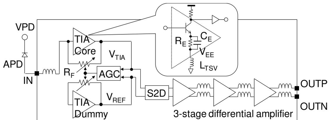
Fig. 2: Block diagram of 25G BTIA.
