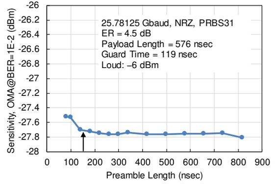
Fig. 8: Settling time of BM-Rx.
