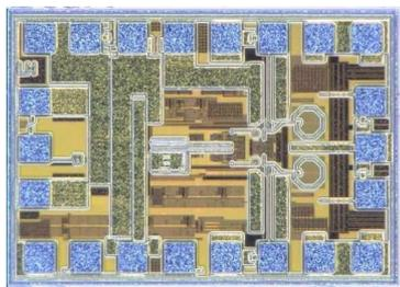
Fig. 3: Chip photograph ( $1.31 \times 0.92 \text{ mm}^2$ ).
