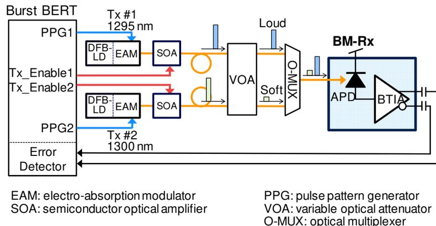
Fig. 6: Setup for burst BER measurement of BM-Rx.
