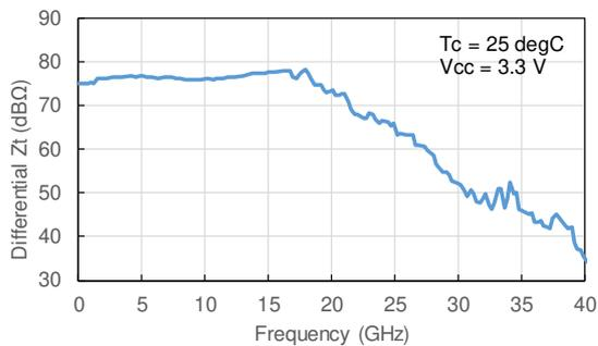
Fig. 4: Frequency response of BTIA.
