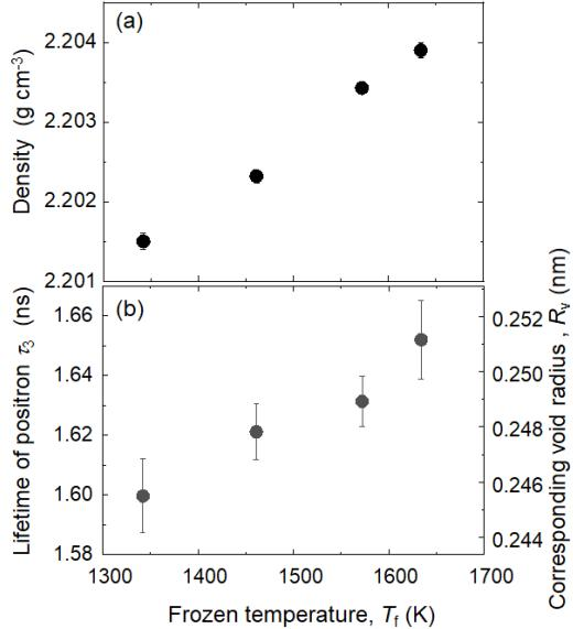
Fig. 2 (a) Density and (b) Lifetime of positron,  $\tau_3$  and corresponding void radius against fictive temperature in silica glass [6].
