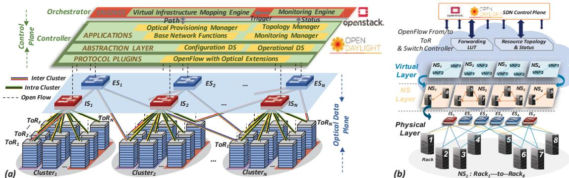
Fig. 1: (a) Reconfigurable SDN-enabled optical DCN. (b) NS allocation over infrastructure.
