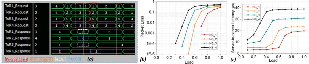
Fig. 3: (a) Flow control signals monitored switch controller. (b) Packet loss (c) latency for 4 NSs with specified priority.
