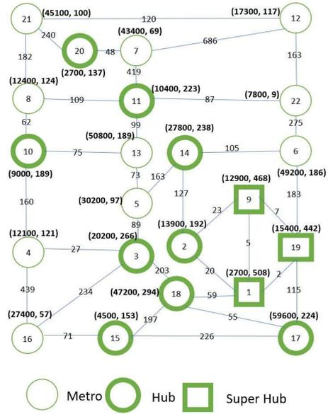
**Fig. 2:** BT-UK network with link length in km, and node metric in parens = (population, dropped wavelength).
