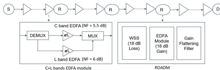
Fig. 1: Multihop path for OSNR estimation.
