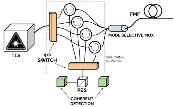
**Fig. 1:** Experimental setup. TLS: tunable laser source, PBS: polarization beam splitter, MUX: multiplexer.
