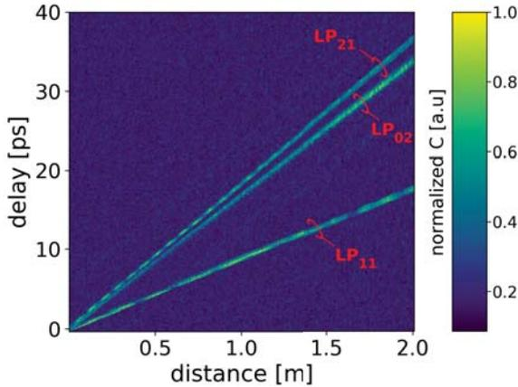
**Fig. 2:** Experimental results for the MD with respect to the  $LP_{01}$  mode group.
