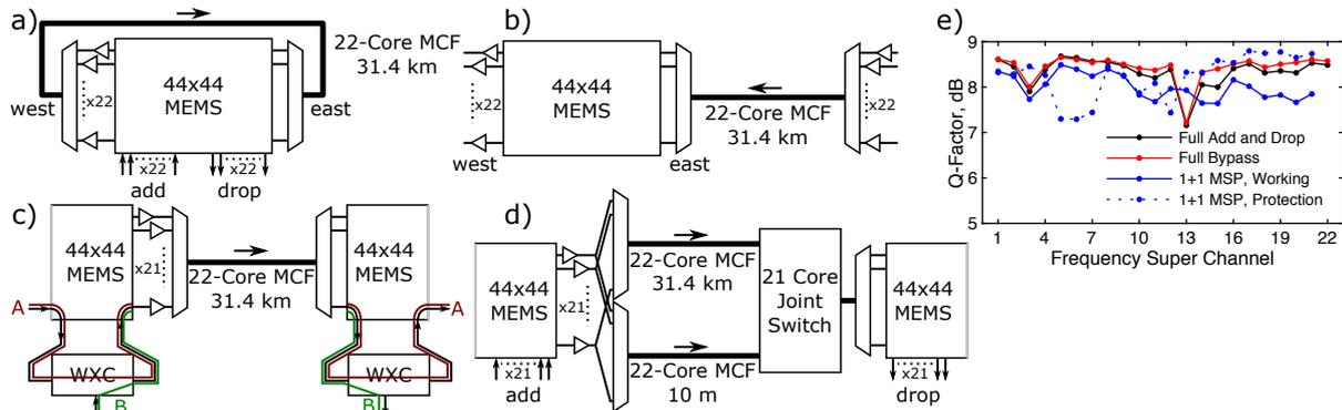
**Fig. 2:** Experimental setup for demonstration of a petabit class SDM network node. a) full spatial add and drop; b) full spatial bypass; c) optical add and drop and optical bypass; d) 1+1 multiplex section protection; e) performance for each scenario.
