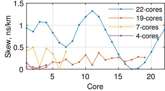
**Fig. 4:** Relative skew in 4, 7, 19 and 22-core MCFs.
