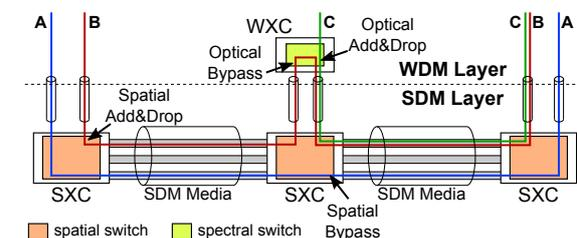
**Fig. 1:** Simplified diagram of a hierarchical SDM network.
