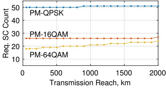
**Fig. 3:** Required number of spatial channels for 1 Pb/s transmission versus the transmission reach.
