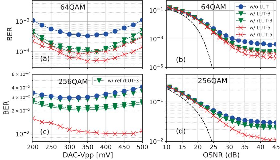
**Fig. 3:** BER versus DAC- $V_{pp}$  (a), (c) and OSNR (b), (d) for 64 and 256 QAM respectively. rLUT: reduced-size LUT, ref rLUT: reduction scheme after<sup>[5]</sup>
