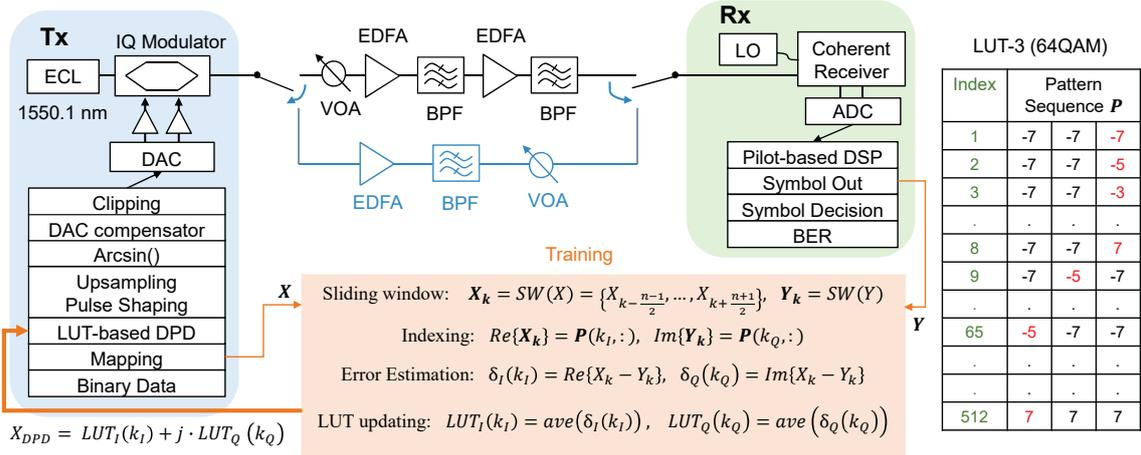
Fig. 1: Experimental setup and block diagram for LUT implementation.
