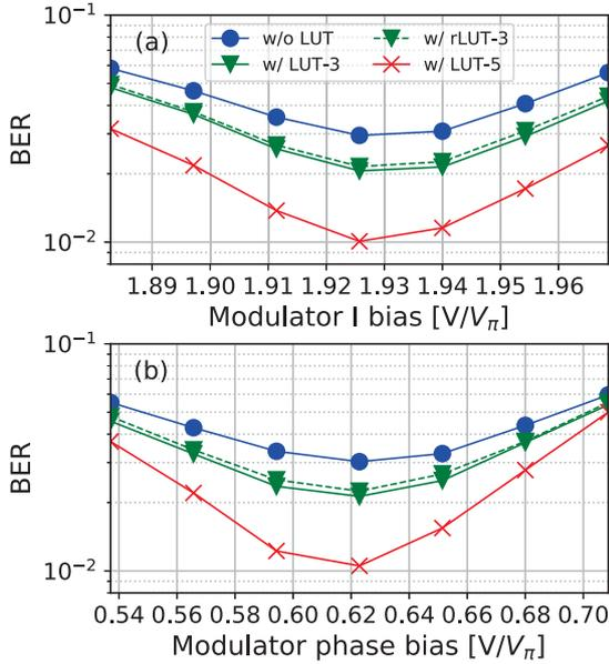
**Fig. 4:** BER versus (a) modulator I bias, (b) modulator phase bias for 256QAM. rLUT: reduced-size LUT.
