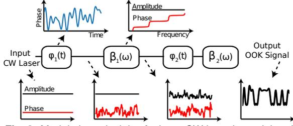
**Fig. 2:** Modulation principle: An input CW-laser is modulated to a binary on-off keying (OOK) signal using two stages<sup>[8]</sup>.
