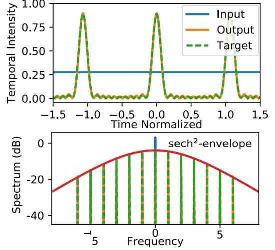
**Fig. 3:** Simulated bandwidth limited frequency comb with Sech<sup>2</sup> envelope with 13 lines generated from input CW laser using 11 stages<sup>[11]</sup>.
