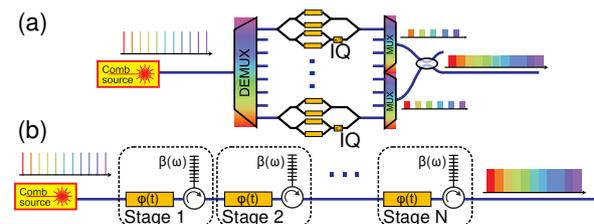
**Fig. 1:** (a) Schematic of a traditional comb-based WDM system using a DeMUX-MUX combination and N independent MZM-based IQ-modulators. (b) Proposed multi-channel modulator using multiple cascaded stages of temporal and spectral phase modulation to simultaneously modulate each input line with an independent waveform.
