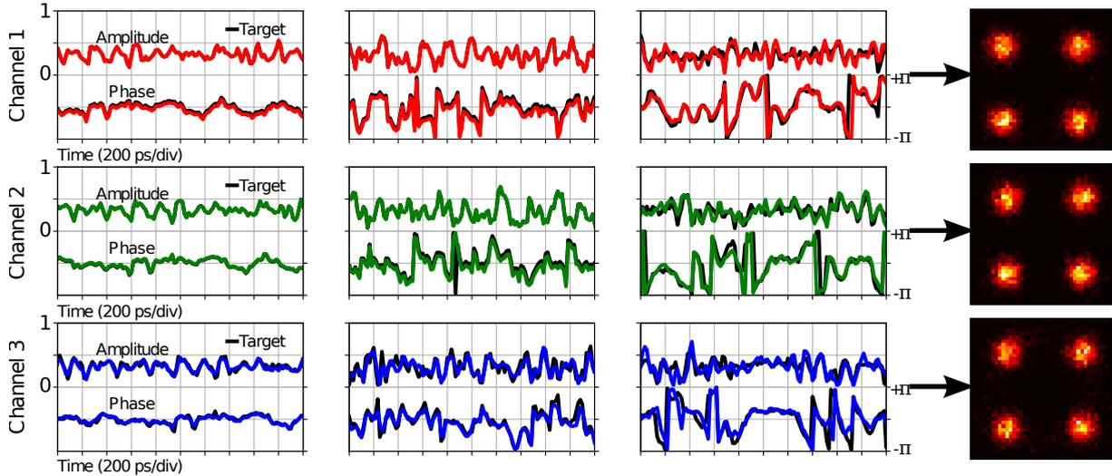
**Fig. 4:** Measured output waveforms simultaneously modulated onto three lines originating from a frequency comb without the use of a DeMUX-MUX combination<sup>[9]</sup>. The transformation was implemented with 8 stages and the output signals are shaped with a 1% roll-off root-raised cosine filter.
