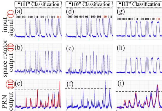
**Fig. 3.** (a) Time traces from the experimental evaluation of 3-bit classification with space rotation mask: (a)-(c)  $m_t="000"$  and (d)-(f)  $m_t="001"$ . (h)-(i) depicts results for a mask of  $m_t="000"$  using NRZ data. y-axis: (2.90mV/div), (a)-(f) x-axis: (980psec/div), (g)-(i) x-axis: (500psec/div).
