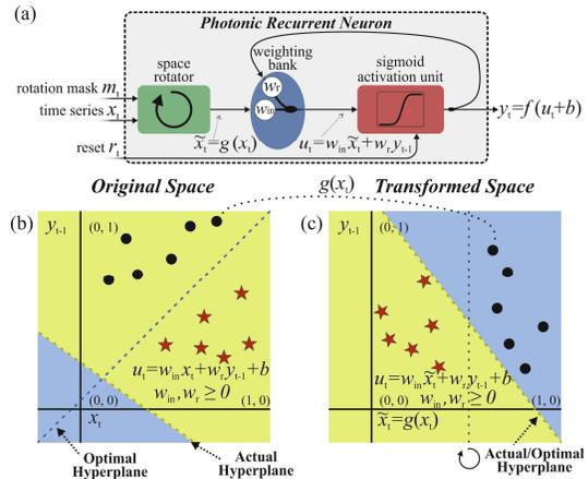
**Fig. 1.** (a) Layout of the proposed PRN, (b) the original sample space that supports positive weights and (c) the transformed sample space.
