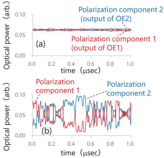
**Fig. 4:** Polarization components of the pump light measured at OE1 and OE2: (a)  $\Delta L$  was optimized, (b)  $\Delta L$  was not optimized.
