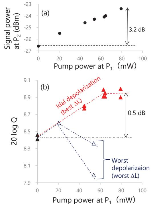
**Fig. 5:** Transmitted signal at various pump powers: (a) measured signal power at  $P_2$ , (b) measured Q factor.
