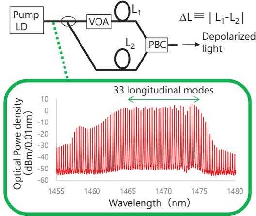
**Fig. 2:** Construction of the dual-arm depolarizer and optical spectrum of the pump light.
