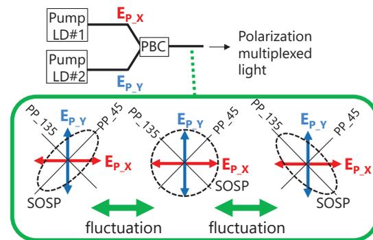
Fig. 1: Synthesized polarization generated using a two-pump light source.
