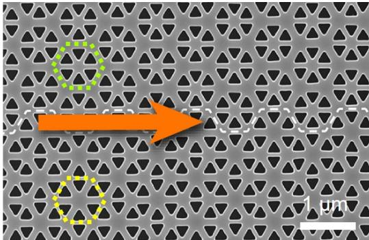
**Fig. 1:** Topological photonic crystal exhibiting the quantum spin Hall effect for light. The edge (white dashed line) separates two domains with differing bandstructure topology. The crystal structure is differentiated by the fact that the holes in the hexagonal unit cell are either closer together (green, ‘shrunken lattice’) or further apart (yellow, ‘expanded lattice’). This deformation opens a bandgap on either side of the edge, which in turn supports a topological edge state.
