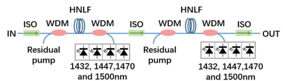
Fig. 1: Structure of the C+L band lumped Raman amplifier
