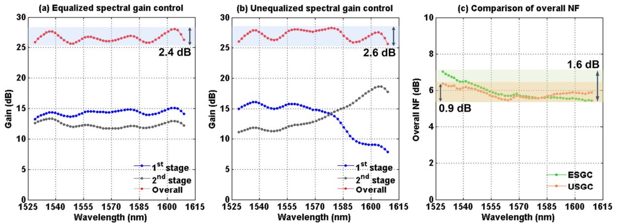
**Fig. 3:** Gain profiles of the dual-stage LRA under (a) ESGC conditions or (b) USGC conditions; (c) Comparison of the overall NF between the two schemes
