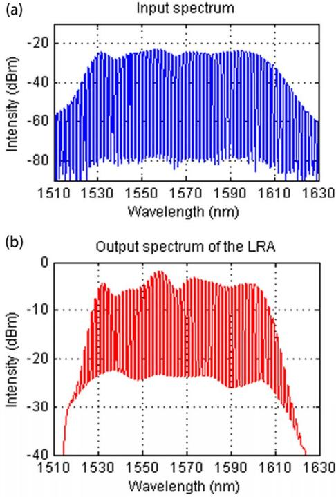
**Fig. 2:** Spectra recorded at both (a) input and (b) output of the LRA (operated with USGC) (resolution: 0.2 nm)
