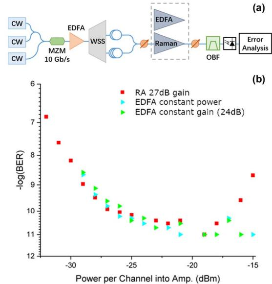
**Fig. 4:** (a) Schematic of the back-to-back BER test and (b) the performance of the LRA compared with EDFAs
