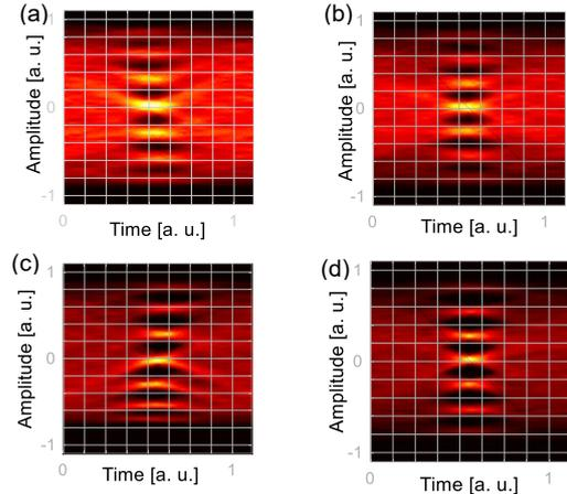
**Fig. 5:** Eye diagram after FFE for 1334.5nm at -3dBm
