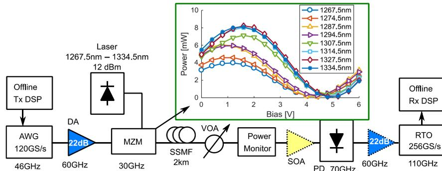
**Fig. 2:** Experimental setup. Inset: MZM characteristics. DSP: digital signal processing, AWG: Arbitrary Waveform Generator, DA: Driver Amplifier, VOA: Variable Optical Attenuator, SOA: Semiconductor Optical Amplifier, PD: Photodetector, RTO: Realtime Osc.
