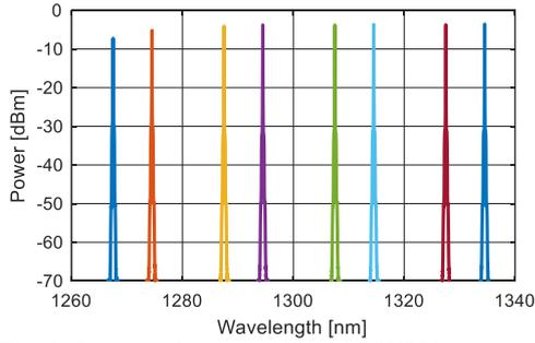
**Fig. 1:** Spectra of the modulated 8 MWDM wavelengths
