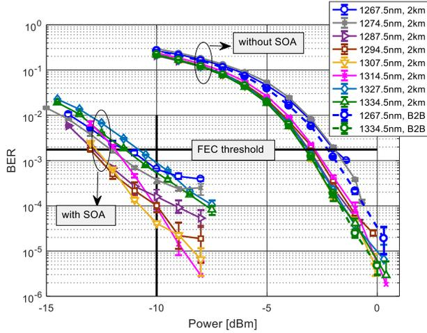
**Fig. 4:** BER vs power for the 8 wavelengths
