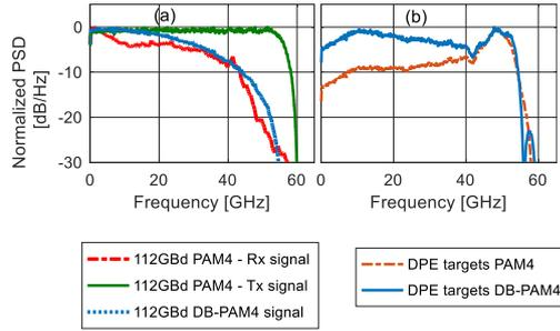
**Fig. 3:** (a) Tx, Rx and DB-PAM4 PSD, (b) Tx PSD with DPE
