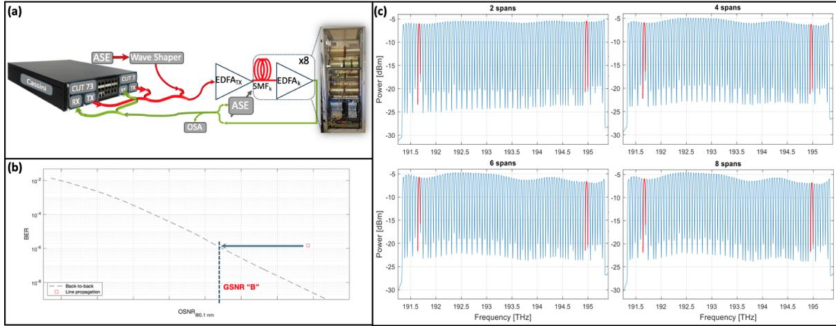
**Fig. 2:** (a) Experimental setup, (b) GSNR "B" evaluation method, (c) received WDM comb spectra for different line lengths.
