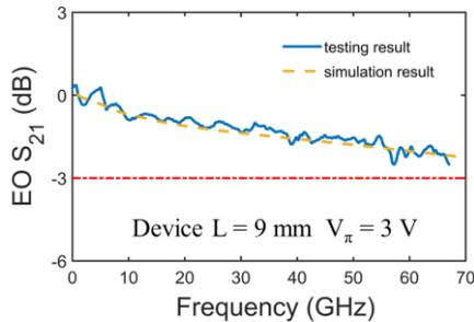
**Fig. 3:** Measured EO frequency response of the 9-mm-long modulator.
