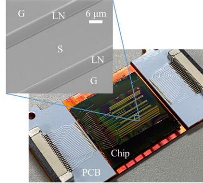
Fig. 2: Optical image of fabricated chip. The inset is the SEM image of TWE formed in GSG configuration.
