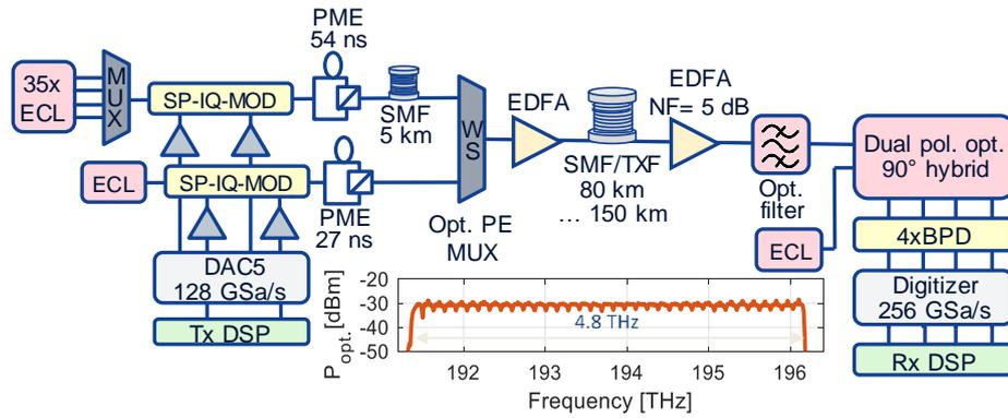
**Fig. 2.** Experimental setup of 36 channel WDM experiment. The inset shows the optical spectra allocating 4.8 THz in total.
