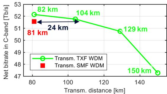
**Fig. 6.** Net bitrate in C-band versus transmission distance for SMF and TXF fiber transmission.
