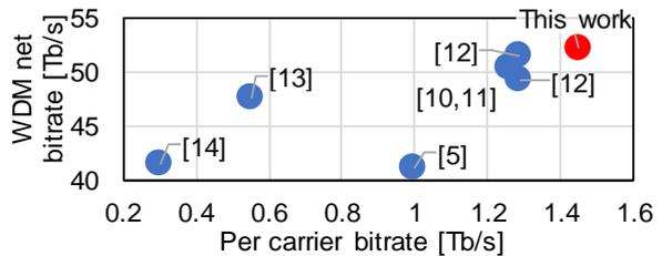
Fig. 1. Reported WDM net bitrates vs. per carrier bitrate. The red marker shows this work.
