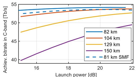
**Fig. 3.** Achievable bitrate in C-band versus launch power for transmission over TXF fiber over different distances.
