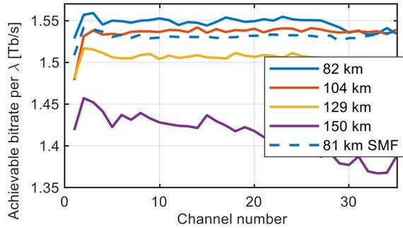
**Fig. 4.** Achievable bitrate per  $\lambda$  for optimum launch power at each transmission distance over TXF fiber.
