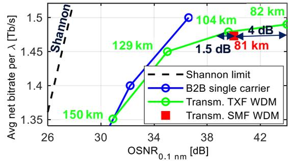
**Fig. 5.** Average net bitrate after FEC decoding versus OSNR. The OSNR was calculated from received power and EDFAs noise figure.
