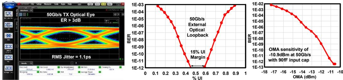
Fig. 6: Measured TX eye (left), measured bathtub curve (middle), and measured receiver sensitivity (right).
