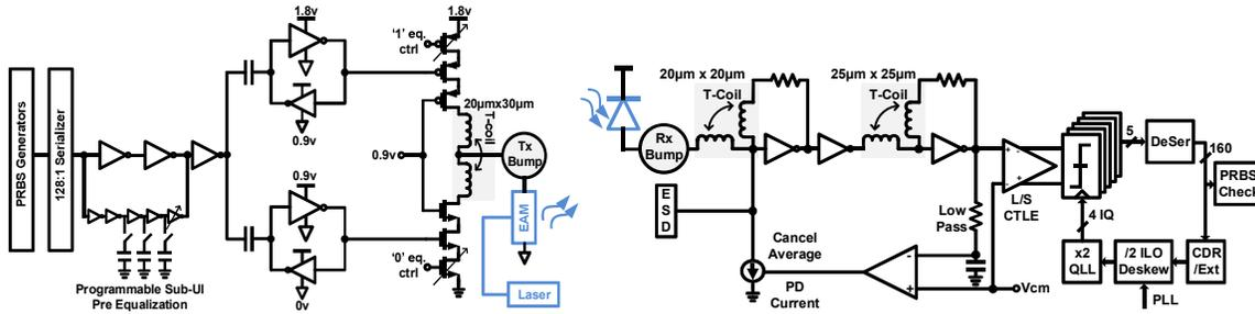
Fig. 5: TX (left) and RX (right) circuit architecture.
