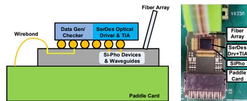
Fig. 1: Optical transceiver over Si-Photonics.
