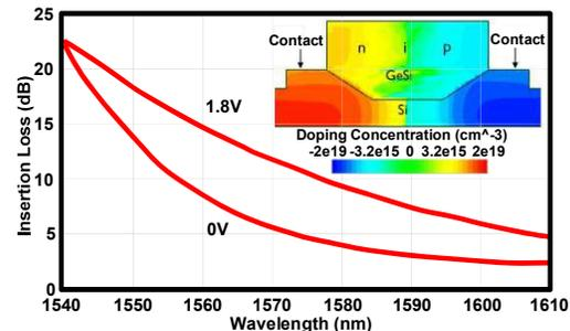
Fig. 2: EAM absorption curves and p-i-n structure.
