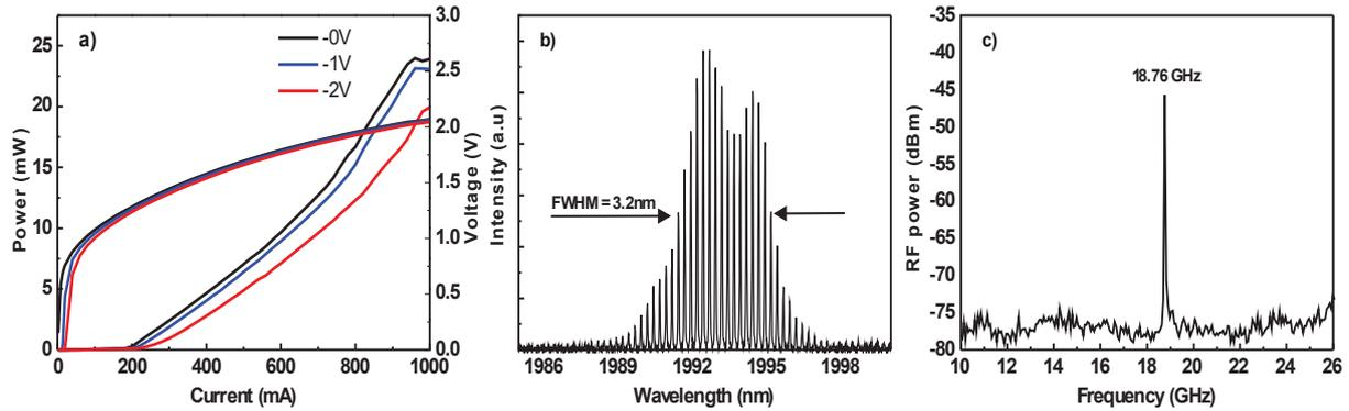
**Fig.2:** a)  $L$ - $I$ - $V$  curve of the laser at room temperature with different  $V_{abs}$ . b) Optical spectrum of the mode-locked laser ( $I_g = 700$  mA,  $V_{abs} = -2$  V). c) RF spectrum of the mode-locked laser ( $I_g = 700$  mA,  $V_{abs} = -2$  V).
